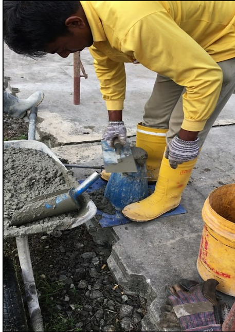
12 th & 13 th August 2018 : - Mock up panel wet joint slum test before casting (on-site)
