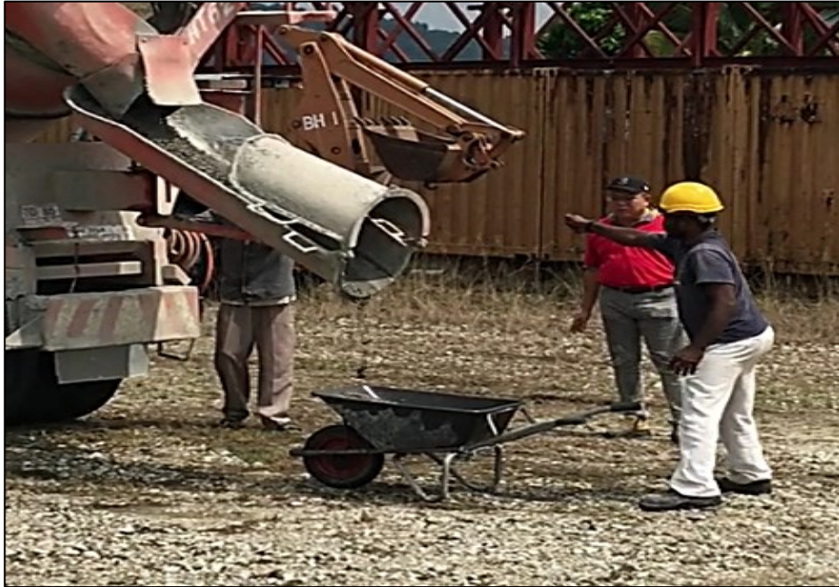
12 th & 13 th August 2018 : - Mock up panel slum test before casting
