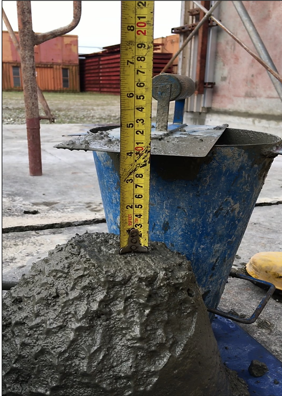
12 th & 13 th August 2018 : - Mock up panel wet joint slum test before casting (on-site)
