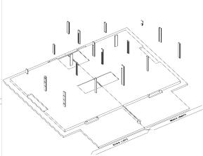
**ROOF LEVEL** Wet Joints (Rebar/Mould/Concrete) = 19 nos. Wet Joints Volume  $= 1.19 m^3$
