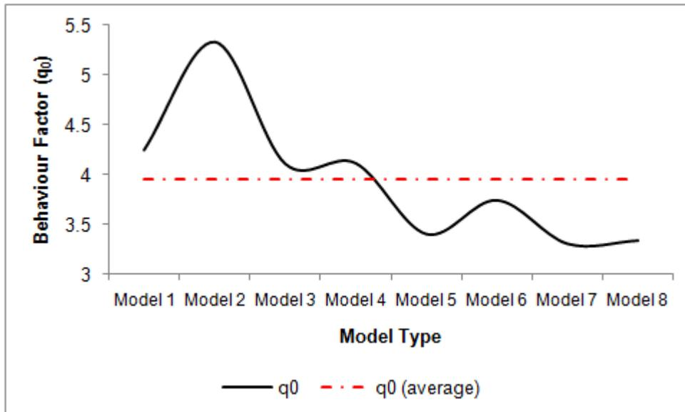
**Figure 3.2.** Behaviour factors of Model 1 to Model 8
