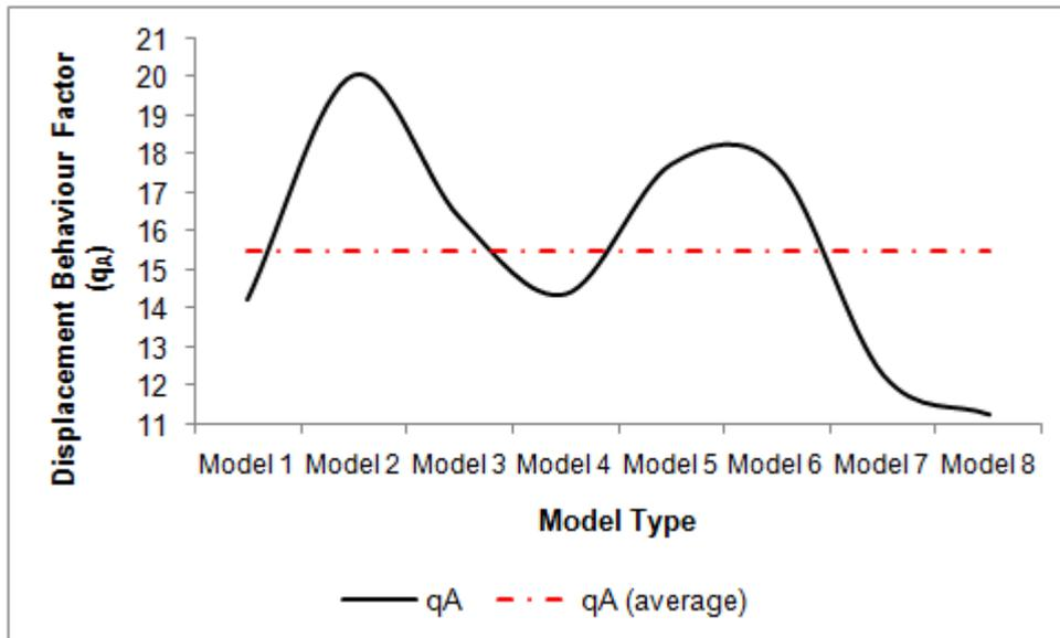
**Figure 3.4.** Displacement behaviour factors of Model 1 to Model 8
