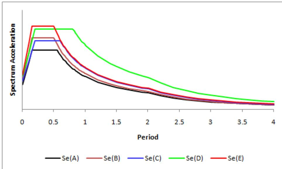
**Figure 2.2.** Design spectra for Malaysia used in pushover analysis for different soil conditions
