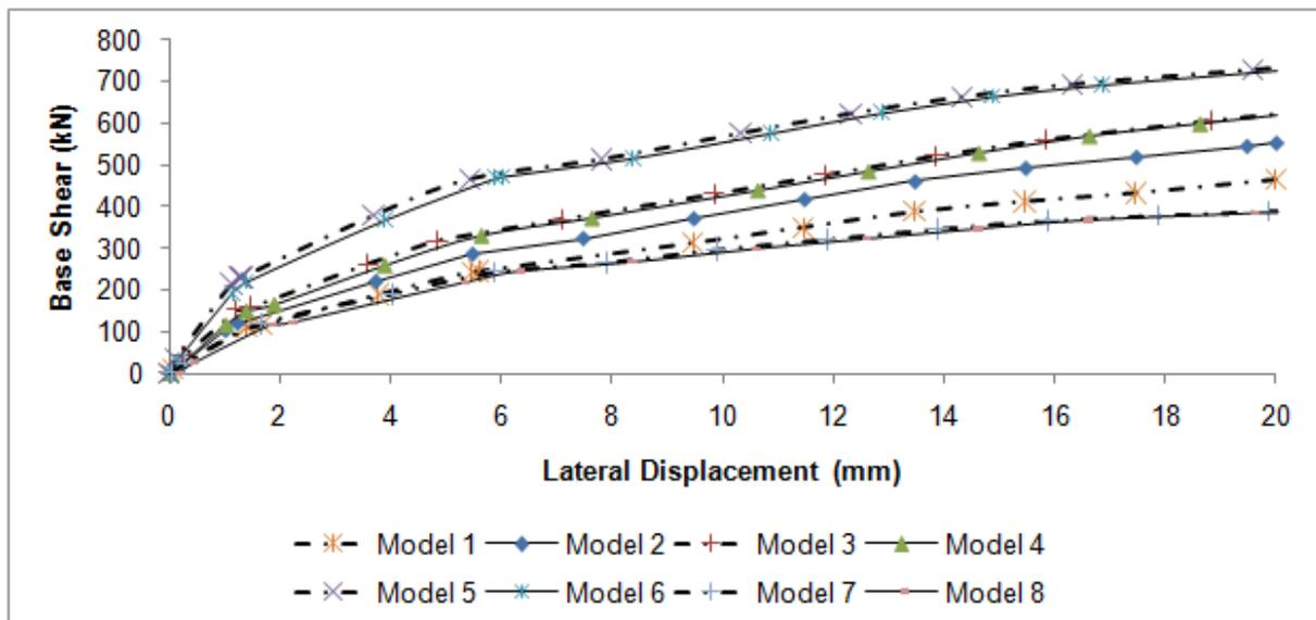
**Figure 3.1.** Pushover curves obtained for Model 1 to Model 8
