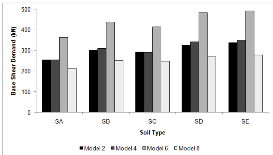
**Figure 3.7.** Base shear demand for different soil condition
